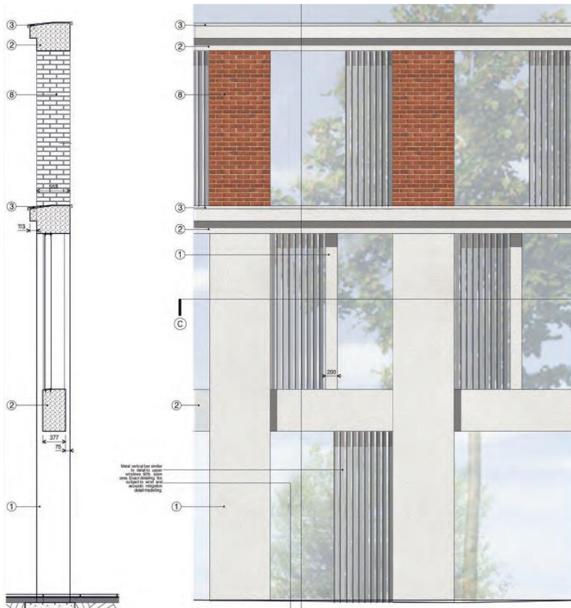
Detailed Elevation of Perimeter Colonnade
