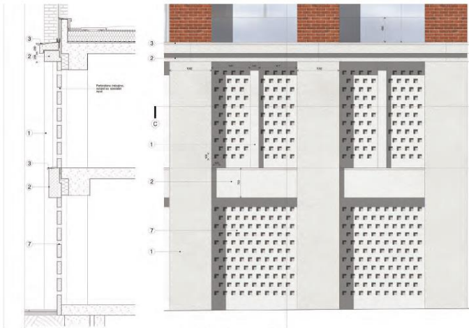
Detailed Elevation of Car Park / Bike stores
